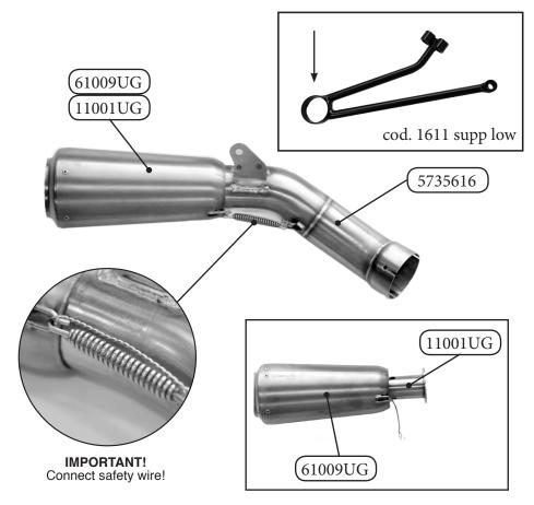
EN Assemble the pipe as pictured below. Remove the rubber ring fom the original passanger frame and place it in the subframe (cod. 1611 supp low) Do not forget to connect the safety wire!
