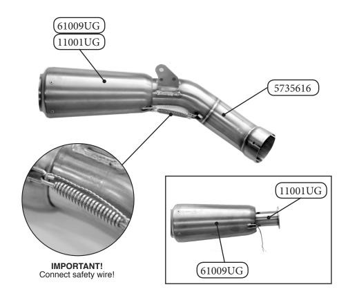
**EN** Assemble the pipe as pictured below. Connect to the mounting point on the passenger frame. Do not forget to connect the safety wire!
